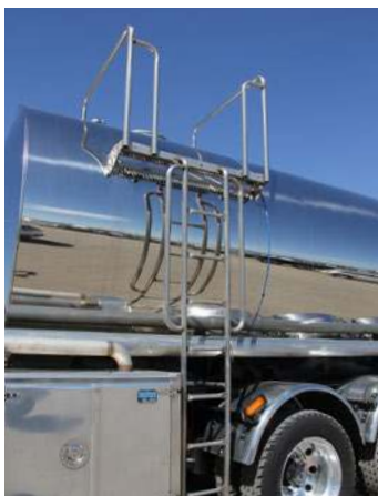
Top access with stainless steel ladder, platform and hand rails.
