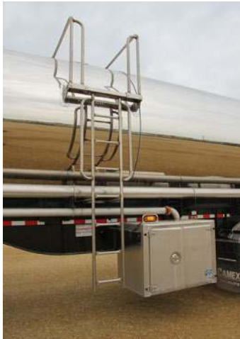
Heavy-Duty stainless steel ladder with platform and hand rails.
